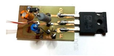
TIP142 regulator with the components mounted on a PC board. All components are mounted on the board with the exception of the 2-amp fuse.
