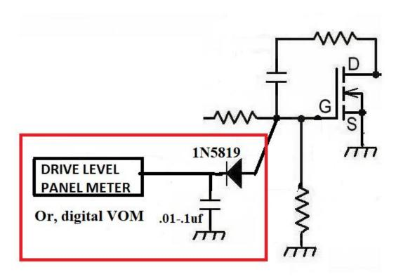
The Drive Level circuit consist of a 1N5819 connected to the MOSFET Gate. The circuit does not load down the gate drive, so it can be connected to the gate to monitor the drive in real time or during testing and setup.
