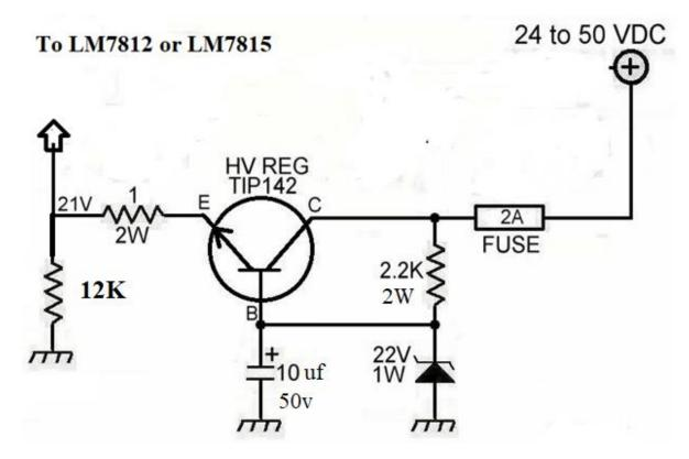
The TIP142 is rated at 100V, 10A, 125-watt dissipation. This makes it a very rugged device for a regulator.
